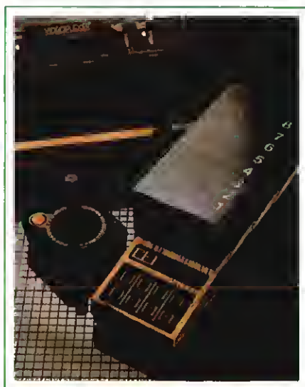
The Videoplexer from Compro Electronics holds up to eight videogame cartridges.
